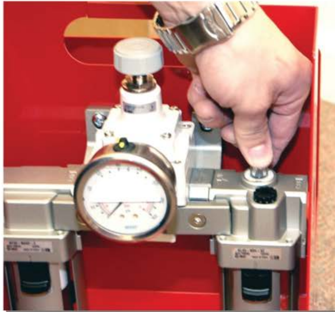
Figure 19. Adjusting FRL Oil Flow
