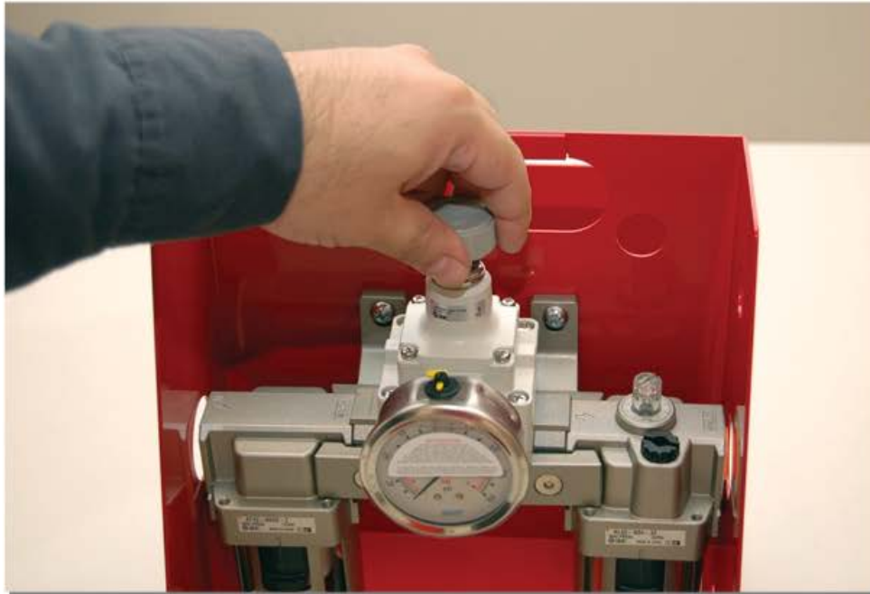
Figure 18. Adjusting FRL Regulator
