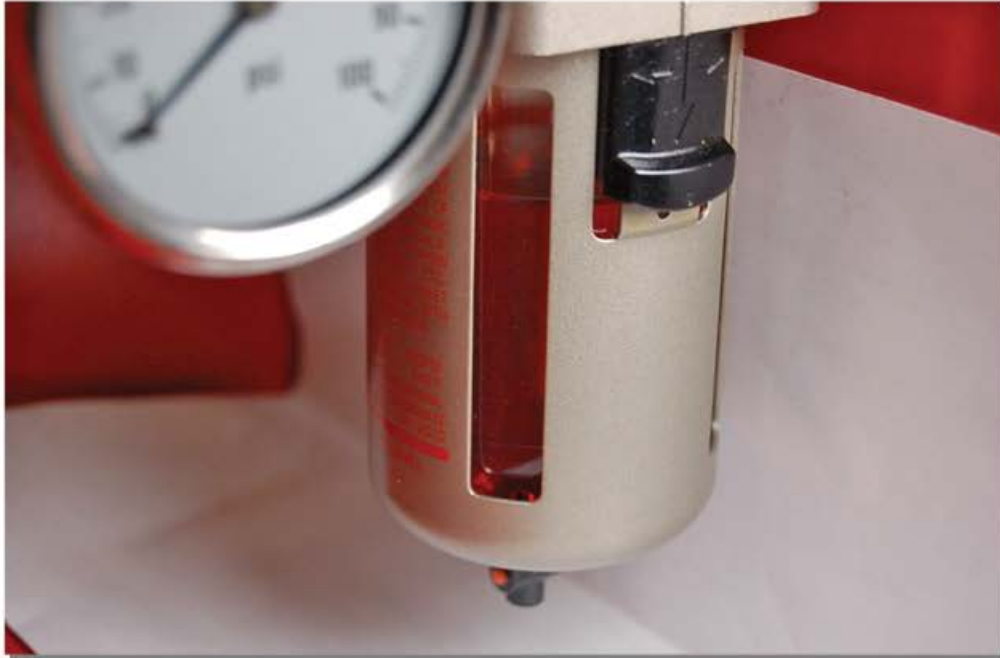
Figure 17. FRL Unit – Lubricator 2/3 Full of Oil
