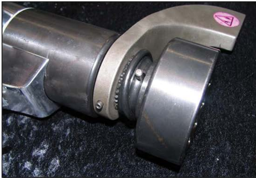
Figure 7. Installing Socket Locking Pin and Retaining Ring
