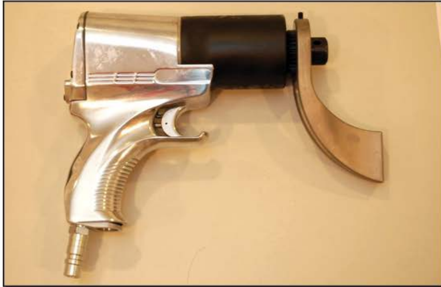
Figure 4. Reaction Arm installed
