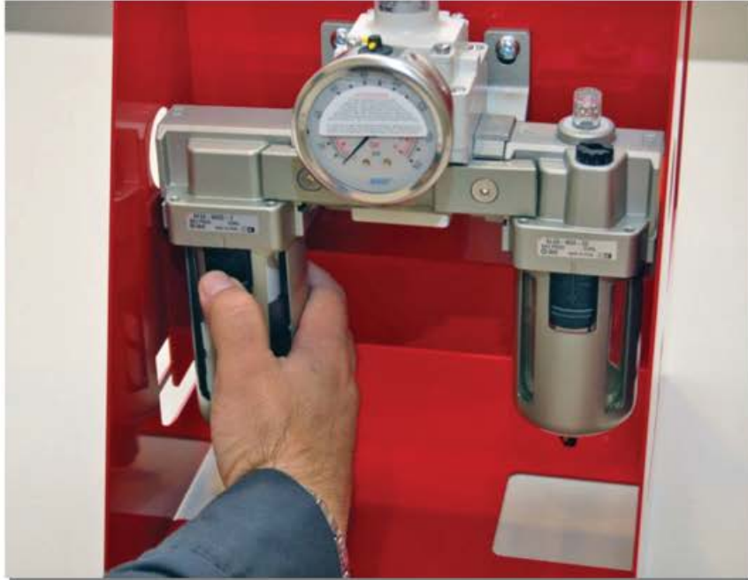
Figure 15. Emptying the FRL Filter Reservoir
