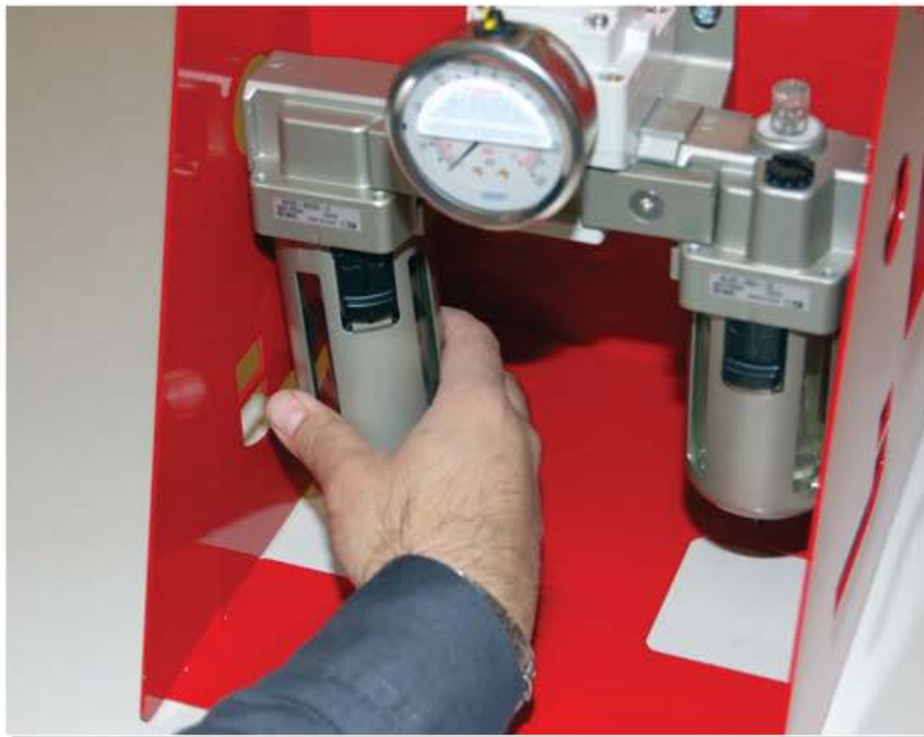
Figure 16. Detaching FRL Reservoir
