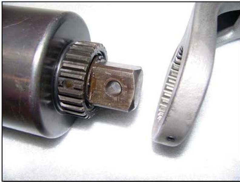
Figure 3. Installing a Reaction Arm
