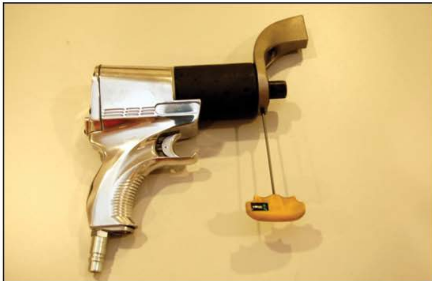
Figure 5. Tightening Reaction Arm Set Screw
