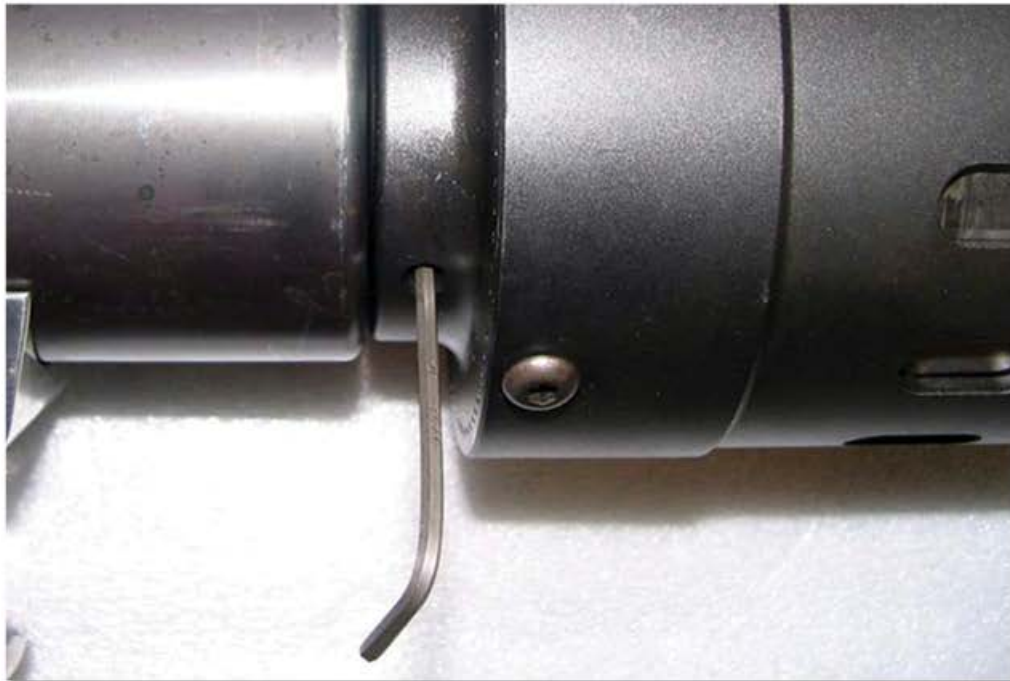
Figure 25. Tightening HYTORC Washer Set Screw
