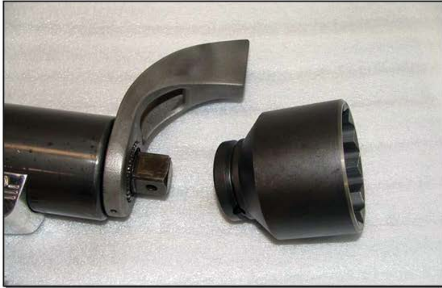
Figure 6. Installing jGun Socket
